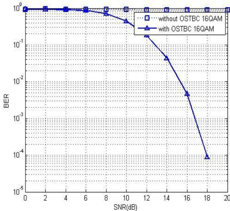
Fig. 5: BER comparison for 16-QAM
