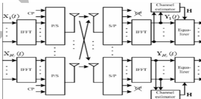
Fig. 2 MIMO OFDM system with Alamouti
