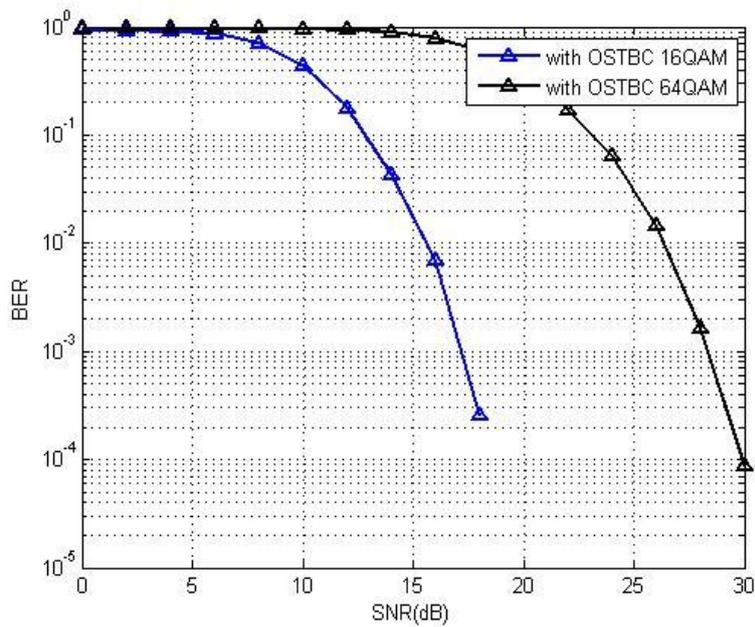
Fig.7: BER comparison of 16 QAM and 64 QAM for OSTBC
