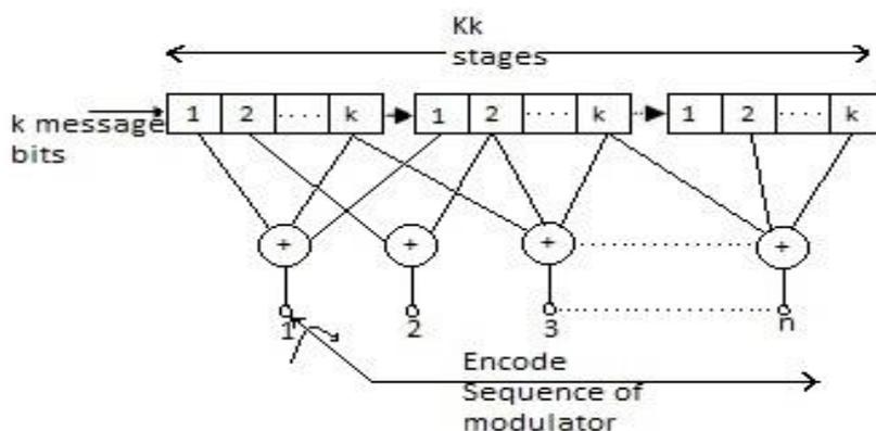
Fig. 3: Convolutional Encoder
